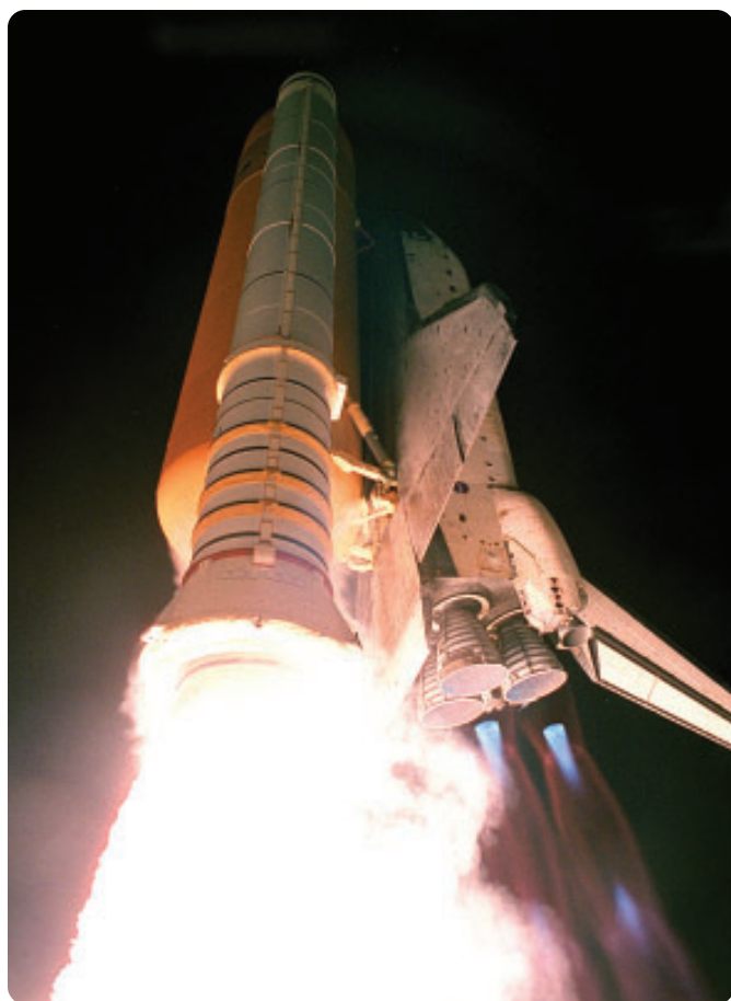
Figure 1 The main engines of the space shuttle react liquid hydrogen with liquid oxygen to provide thrust. Notice the blue flames on the right—this is hydrogen fuel being burned.
