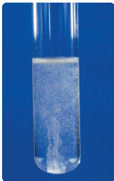
Figure 4 Calcium metal reacts with water to form bubbles of hydrogen gas.
