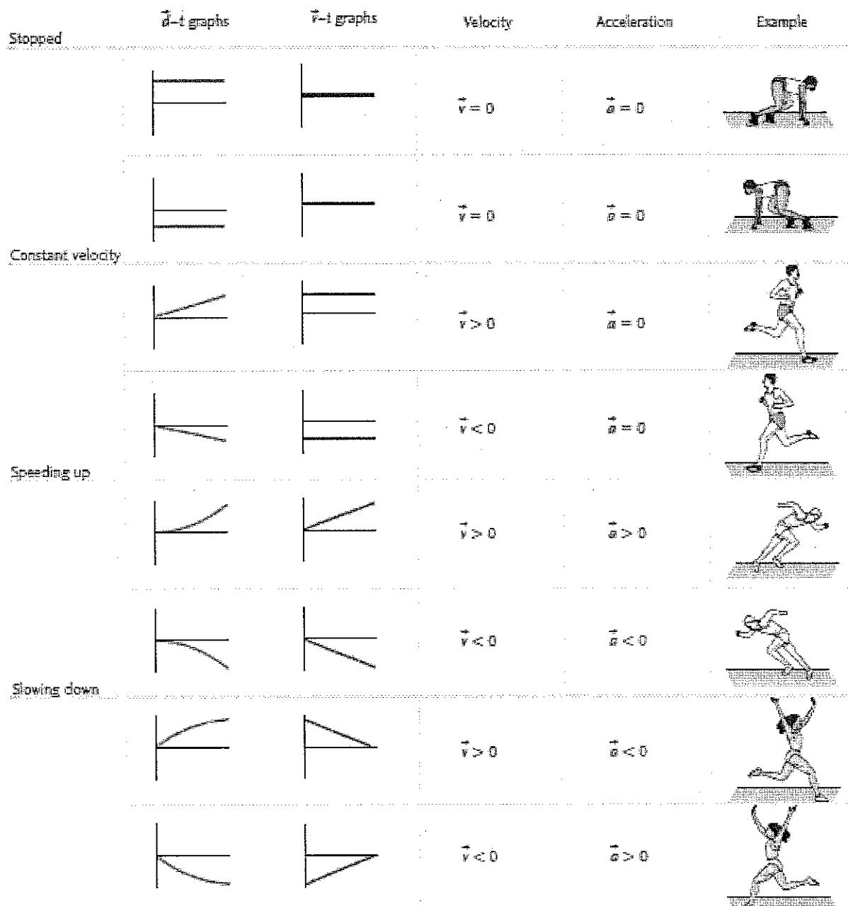
Each  $\vec{v}$ - $t$  graph can be generated from its corresponding  $\vec{d}$ - $t$  graph by taking slopes of the  $\vec{d}$ - $t$  graph at selected times and plotting them on a  $\vec{v}$ - $t$  graph.
