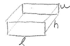
$$V_{\text{rect}} = \text{area of base} \cdot h = l \cdot w \cdot h$$
