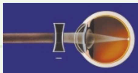
Fig.STSE.11.4 Adding a lens changes the path of incoming light
