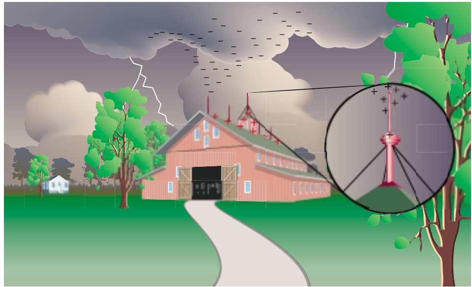
Fig.15.11 A lightning rod prevents a lightning strike
