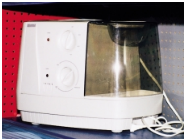
Fig.13.40 An ultrasonic humidifier
