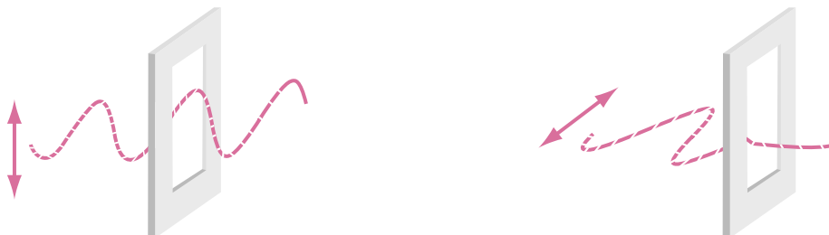
(a) Vertically polarized wave passes through a vertical slit (b) Horizontally polarized wave does not fit through the vertical slit
