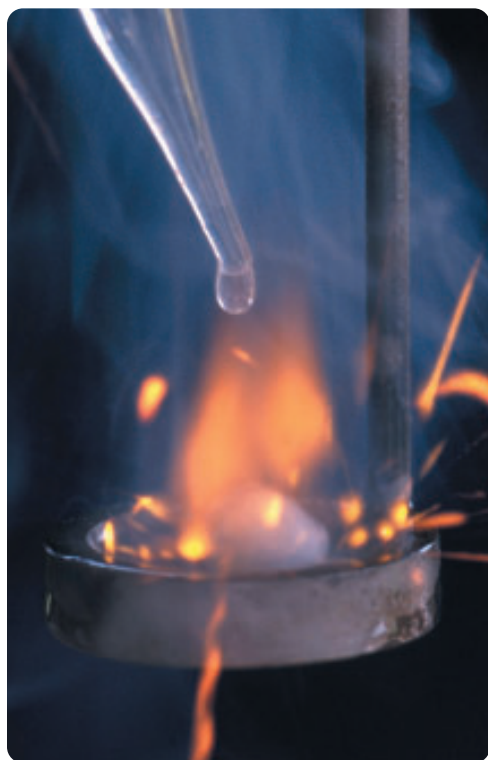
Figure 4 Sodium metal, like all the elements in the Group I column, reacts with water to produce hydrogen gas. The heat that is released in this reaction can ignite the hydrogen.
