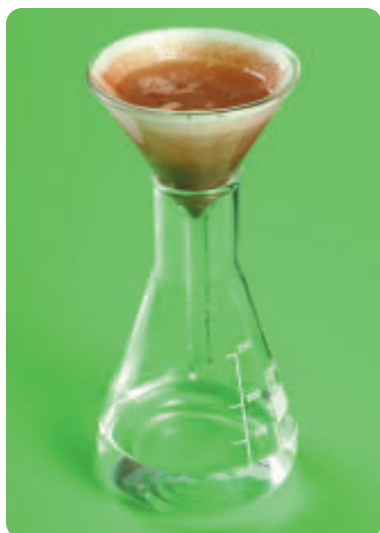
Figure 5 Some substances can be separated from mixtures because of differences in solubility. The brown substance in the photo can be filtered out of the water because the substance is not soluble in water.
